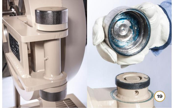
**Step 2:** With the door open, remove the primary O-Ring on the outer periphery of the door [fig 20].
