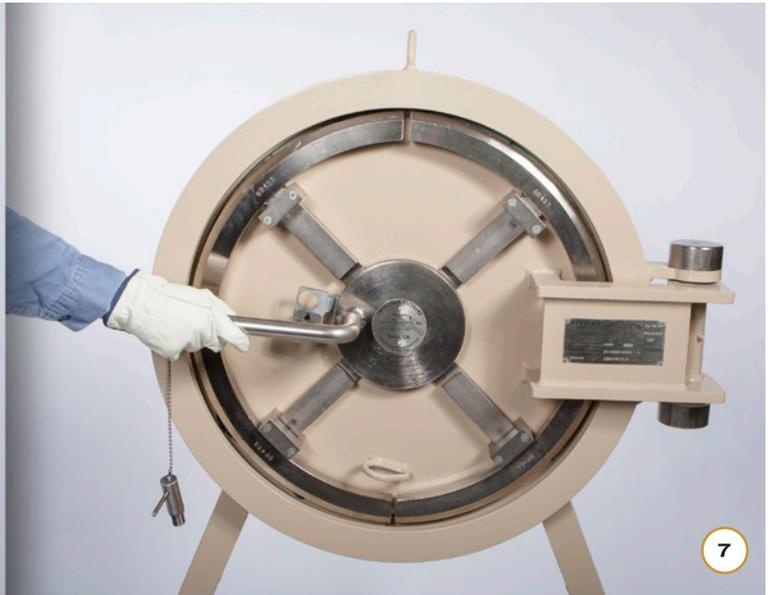
**Step 4:** With door locking lugs disengaged, use door handle to open the door [fig 8], and swing door to open position [fig 9] to gain internal access to vessel.
