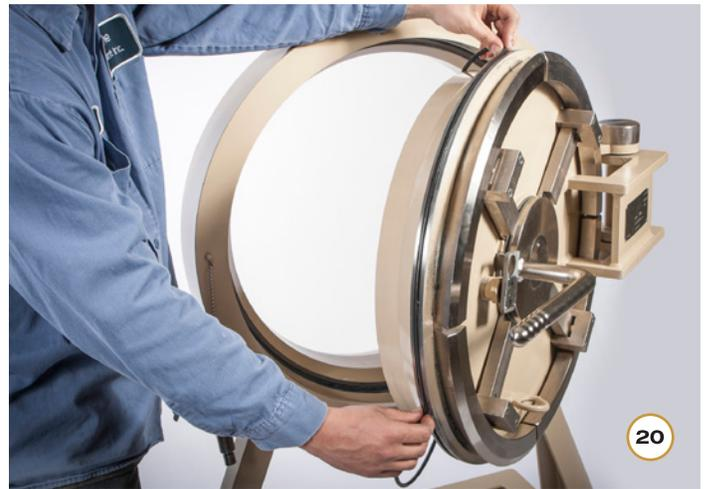
**Step 3:** With O-Ring removed, close the door, do not engage locking lugs. The gap between the outer periphery of the door and inner periphery of the hub can now be viewed and accessed [fig 21].
