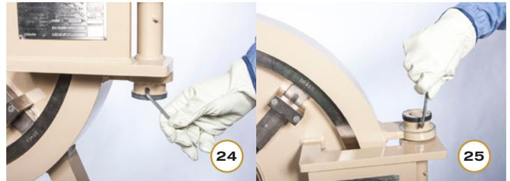
**Step 6:** Make sure all set screws are tight, open and close the door several times to assure there is not door drag on the closure hub.
