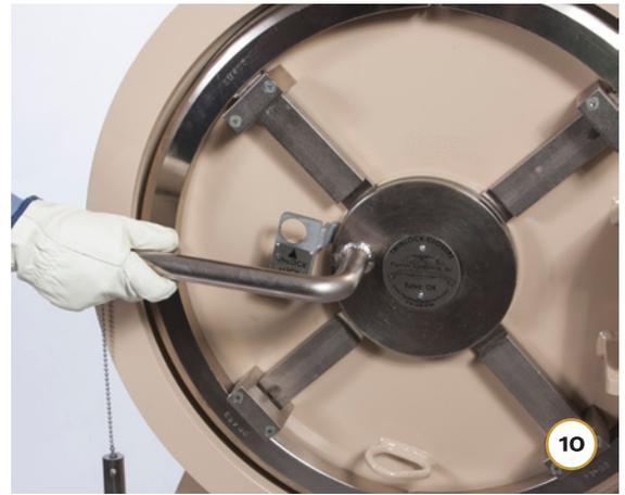
**Step 2:** With the door completely closed, lift door handle to fully engage the door locking lugs [fig 11].
