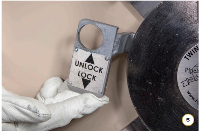
**Step 3:** Standing to the side opposite the door hinge, with Safety Lock in upward position, rotate door handle [fig 6] to disengage the door locking lugs [fig 7].
